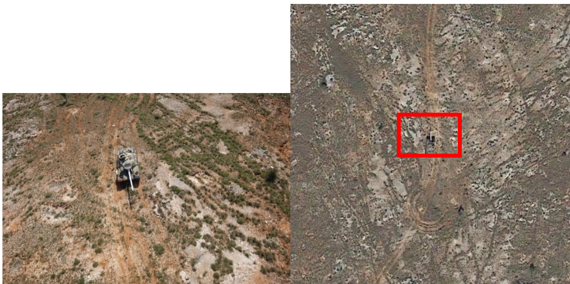
Figure 1: On the left, an example of image taken by the UAV at low altitude and with an oblique view of 30°. On the right, the geo-referenced satellite image of the area with a rectangle showing the footprint of the UAV image.
